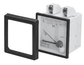
**Ammeters** Type of Protection Ex e II T6 **Certificate of Conformity** PTB No. Ex-87.B.2016U **Approvals** PTB, UL, cUL Movement Moving iron (core) Accuracy 2.5% of range (class 2.5) **Measuring Range** 0-16A direct, C.T. n/1 A **Operating Position** Scale Interchangeable for C.T. n/1 A **Zero Adjustment** At instrument **Terminal Wiring** 2 x 2.5 mm<sup>2</sup> / 14 AWG **Rated Current Marking** Red indicator
