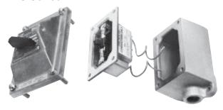
EDS factory sealed snap switches or manual motor starting switches do not need external sealing. The switches are enclosed in a unique sealing well with double flanges which mate with the cover and the body. Small, compact enclosures have accurately ground wide flanges on body, cover and sealing well for flame-tight joints. Wiring pigtails are factory sealed from under the sealing well. Reliable pouring of seals at the factory ensures safe sealing.
