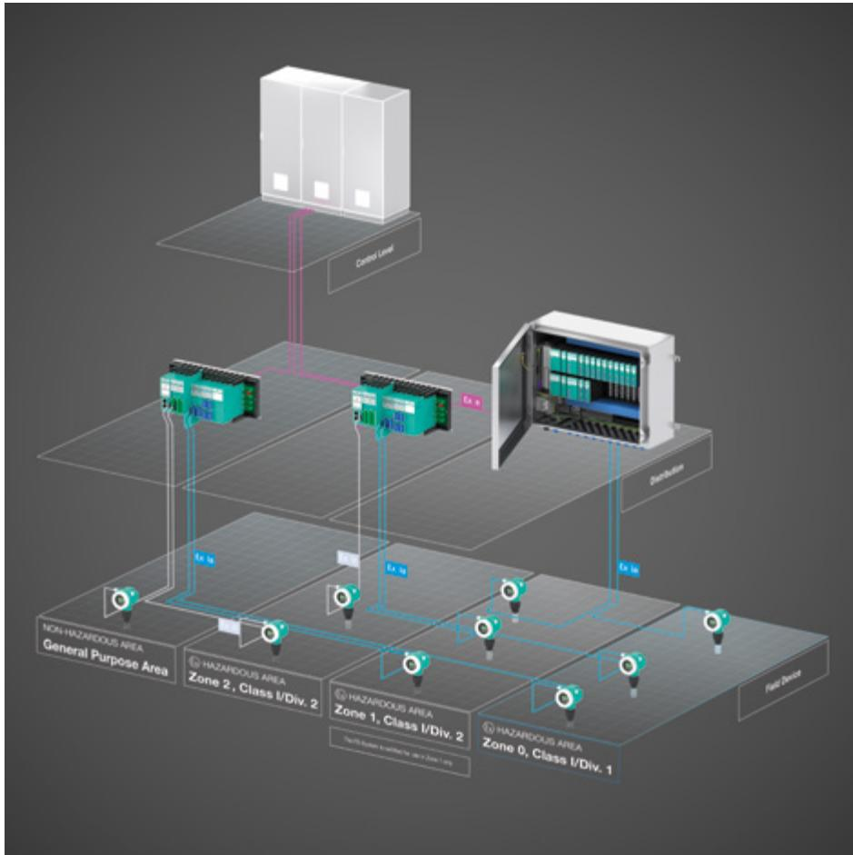
Remote I/O systems combine conventional field technology with modern bus technology. This means that when modernizing and expanding plants, the existing field technology can be connected with the control system over the remote I/O system via a fieldbus.
