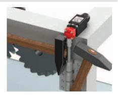
Pin the switch (pin is provided).
