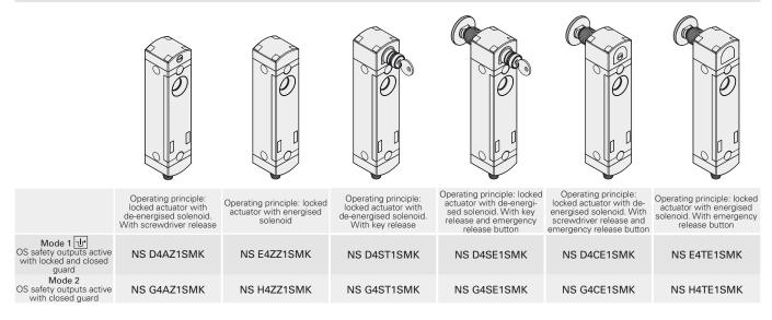
To order a product with lateral connection replace character S with character D in the order codes shown above. Example: NS D4AZ1SMK → NS D4AZ1DMK To order a product with EDM input replace number 4 with number 5 in the codes shown above. Example: NS D4AZ1SMK → NS D5AZ1SMK Legend: <u>u</u> interlock with lock monitoring acc. to EN ISO 14119
