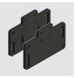
Fixing plate (complete with fastening screws) provided with long slots for adjusting the operating point. Each plate is provided with two pairs of fixing holes, one for standard switches and one for switches with reset device. The actuator thus always has the same actuating point.
